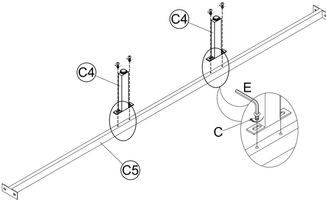
STEP 4: Use Hex Key(E)to tighten Centre Rail(C5)to the Headboard(C7)and Footboard(C6)with Bolt(C)
